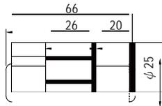
CJ04-1 suitable for 14AWG-16AWG
