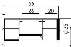
CJ04-1 suitable for 14AWG-16AWG
